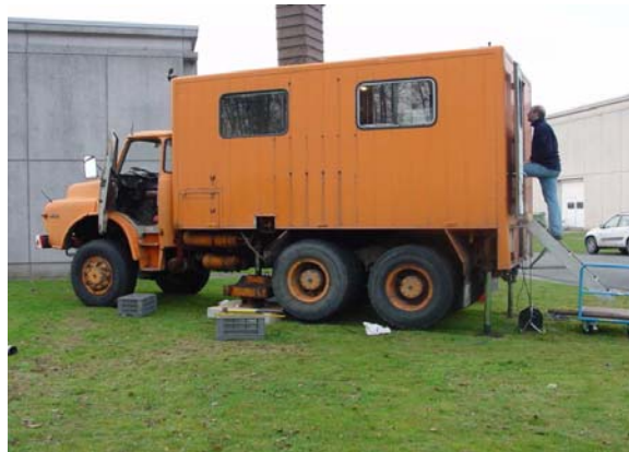
Figure 20. A modified truck for SCPT test (Karl, 2005).
