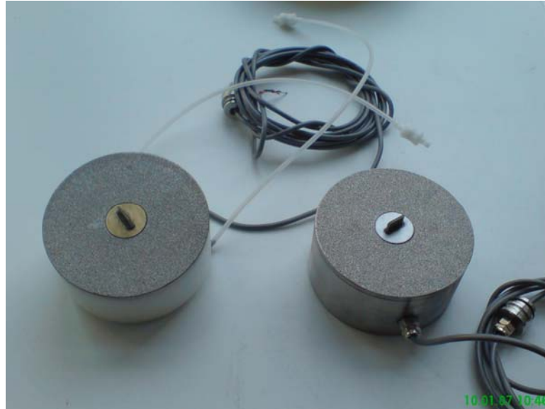
Figure 32. Bender elements installed in top cap and pedestal of a triaxial cell.
